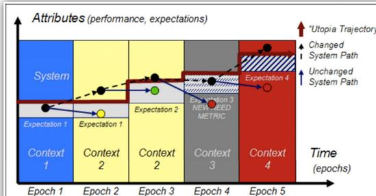
The graph on the left illustrates a five-epoch analysis of a responsive system. An epoch is a discrete time period where **expectations and context** are fixed. A **sequence** of epochs constitutes an era, which is the system lifetime. It is important to note that the **order** of the epochs matters when concerned with the performance of a system.
