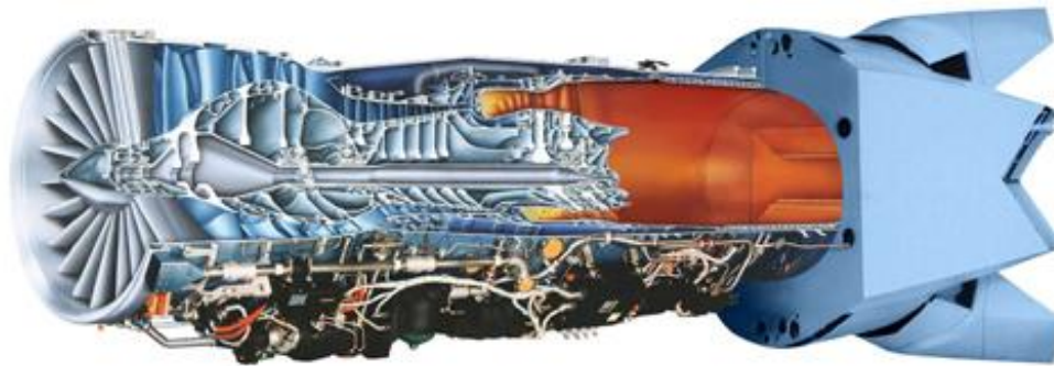
Figure 3. Cutaway of the F119 engine (Pratt & Whitney 2003).
